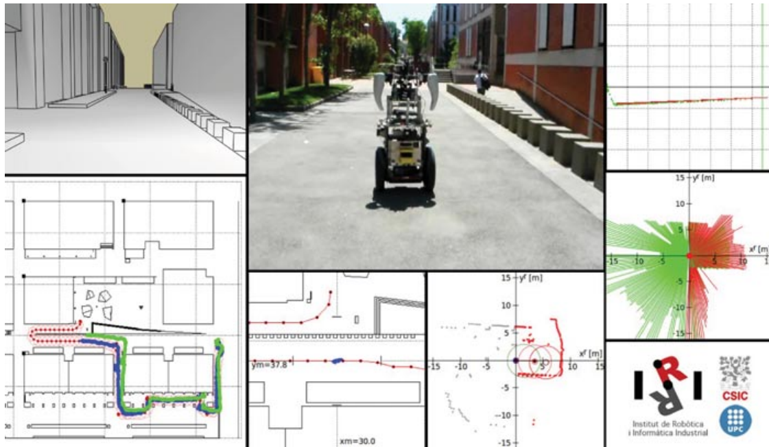
Figure 16. Sample screenshot. Clockwise, starting from the top left: (1) 3D map from the localization viewpoint, (2) handheld camera, (3) vertical laser and regressions, (4) horizontal laser scans in green and expected front laser scan in red, (5) logo, (6) obstacle avoidance and path execution output, (7) path planning output (red) and particle set from the localization algorithm (blue), and (8) path planning (red), accumulated odometry (green), and localization estimate (blue) on the full 2D map, for reference.
