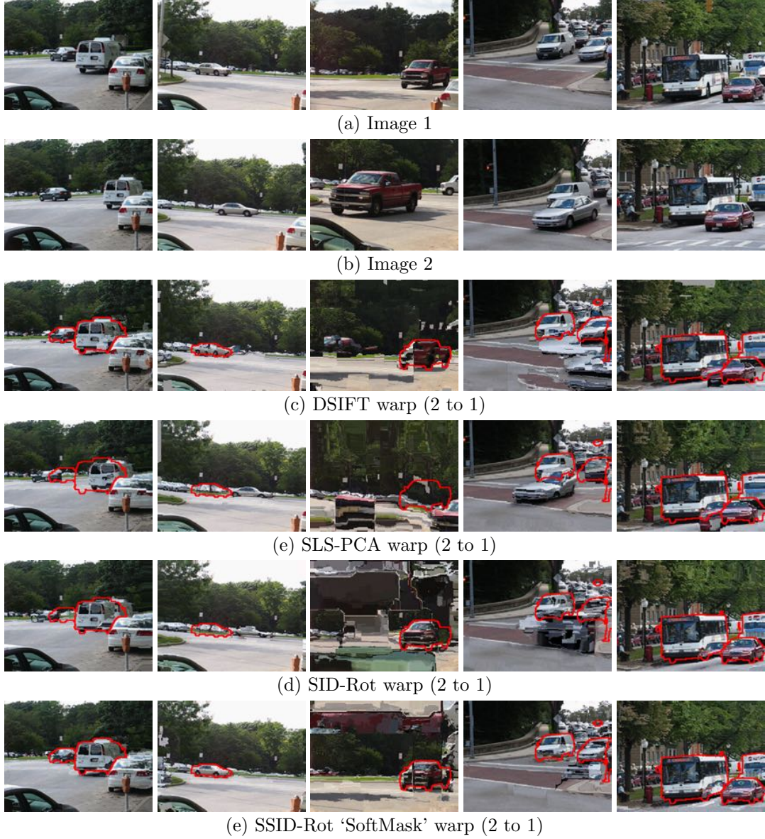
Figure 4.4: Large displacement motion with SIFT-flow, for some of the descriptors considered in this work. We warp image ‘2’ to ‘1’, using the estimated flow fields. The ground truth segmentation masks are overlaid in red: a good registration should bring the object in alignment with the segmentation mask. We observe that segmentation-aware variant SSID does best, with noticeable improvements over its baseline, SID. Similar improvements were observed for SDSIFT over DSIFT.
