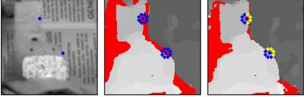
Figure 3.6: Using binary masks to refine the stereo reconstruction of scenes with occlusions, following (Tola et al., 2010). Left to right: reference image, the depth map after the first iteration, and a posterior refinement using the occlusion masks. Enabled grid points are colored blue, and disabled grid points are colored yellow. We show a simplified grid of 9 points with a single ring ( N = 1 ), for simplicity. The images belong to the stereo video dataset of (Sizintsev and Wildes, 2009), extracted with a classical narrow-baseline stereo camera. Occlusion masks become more relevant in wide-baseline setups, for which unfortunately datasets with motion are scarce.
